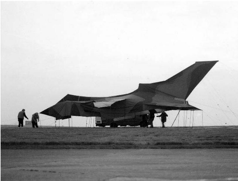
16.9 Textile decoy of a tornado aircraft.
