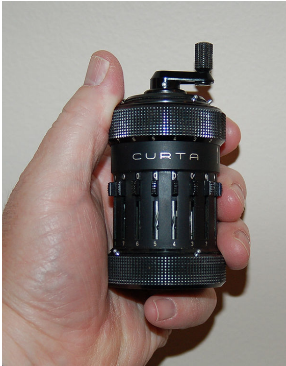
The Curta calculator could also do multiplication and division.
