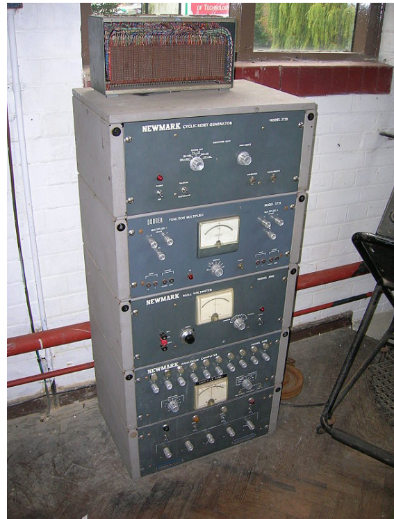
A 1960 Newmark analogue computer, made up of five units. This computer was used to solve differential equations and is currently housed at the Cambridge Museum of Technology.
