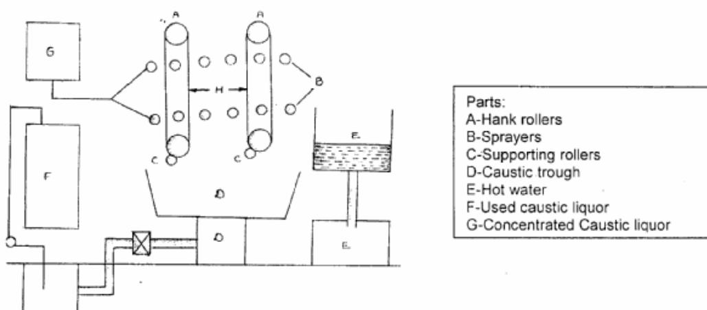
18 to 22% of NaOH is taken in an overhead tank which is the mercerizing liquor. The yarn in hank form is mounted on the two rollers and the tension is applied. The rubber
