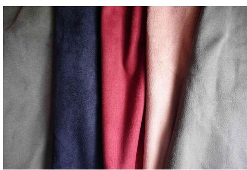
Napping is a process in which a layer of fiber is lifted from the fabric's surface. It creates a pile on top of the fabric. Napping is widely used for knitted and woven fabrics and makes the fabric warmer. The accumulation of piles makes the fabric highly comfortable and soft. Further, it is easy to brush the nap in one direction of the fabric. Some common fabrics on which napping or raising is done are corduroy or velvet fabrics.
